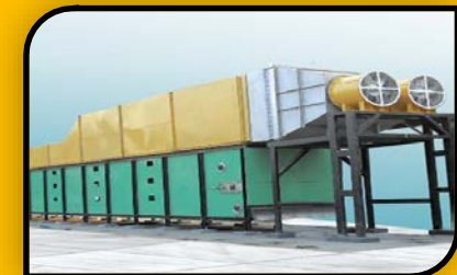
Continuous Mechanised Withering System for Tea Leaf
