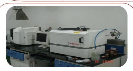
Atomic Absorption Spectrometer & Spark Emission Spectrometer
