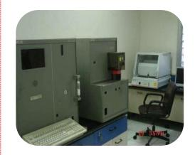
Leco Oxygen Analyzer: R0300 & X- Ray Fluorescence Spectrometer
