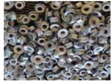
Zinc flake anticorrosive coating for fasteners
