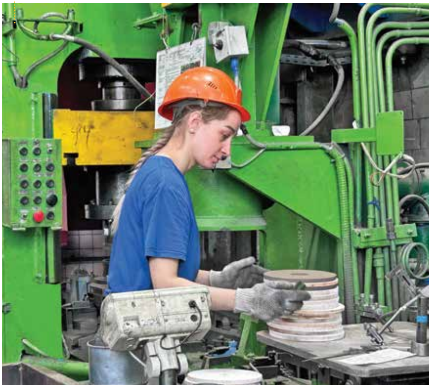
The making of vitrified grinding wheels in VAW
