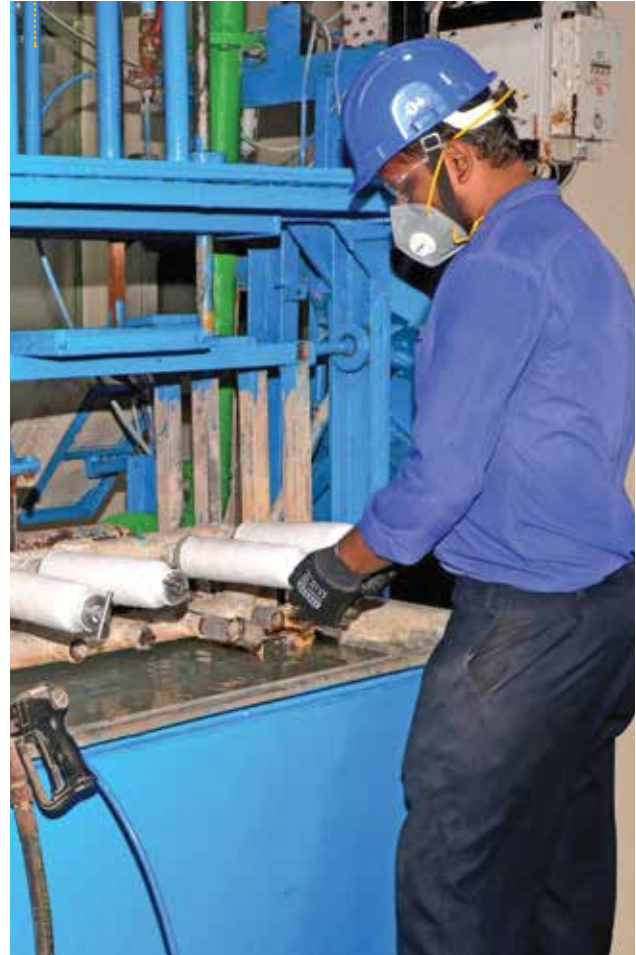
Vacuum forming of ceramic fibre pouring cups
