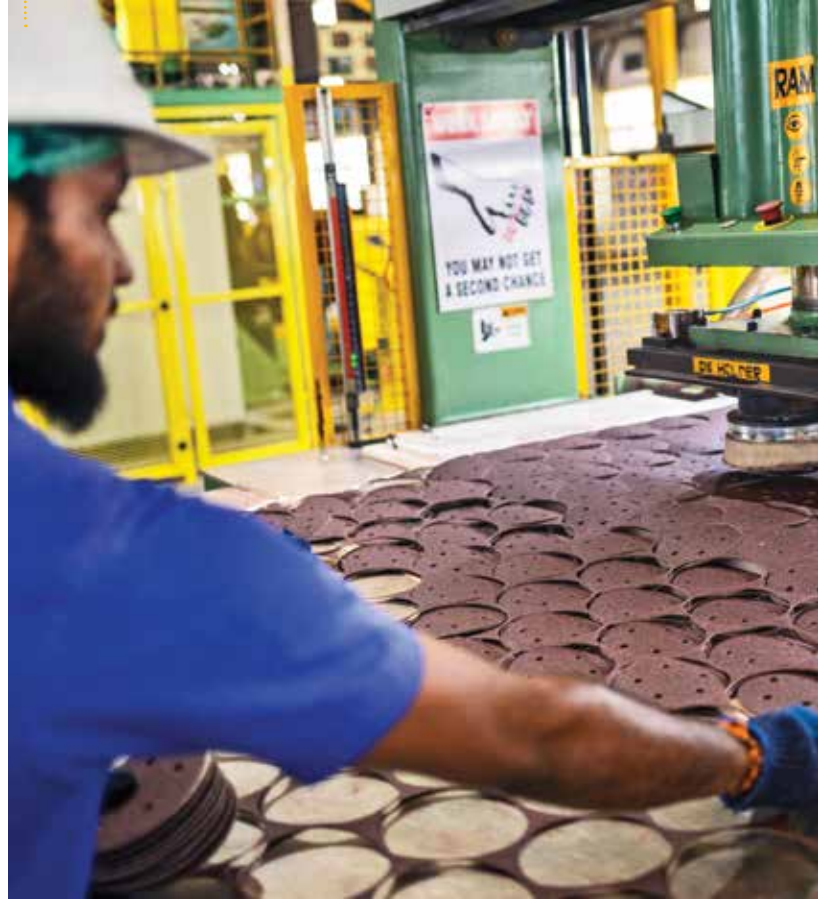
Abrasive discs used for metal, wood and composite applications being punched out at CUMI’s Sriperumbudur facility
