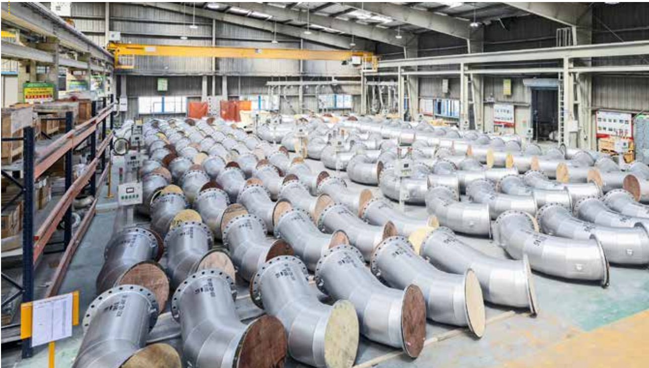
Pre-engineered ceramic lined bends used to convey coal
