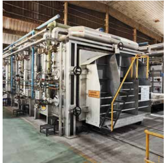
New energy efficient fibre lined kiln for firing glass and super alloy refractories offering a 15% reduction in energy consumption
