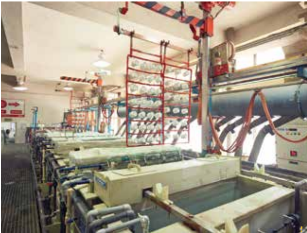
The automatic nickel plating process for metallised ceramics
