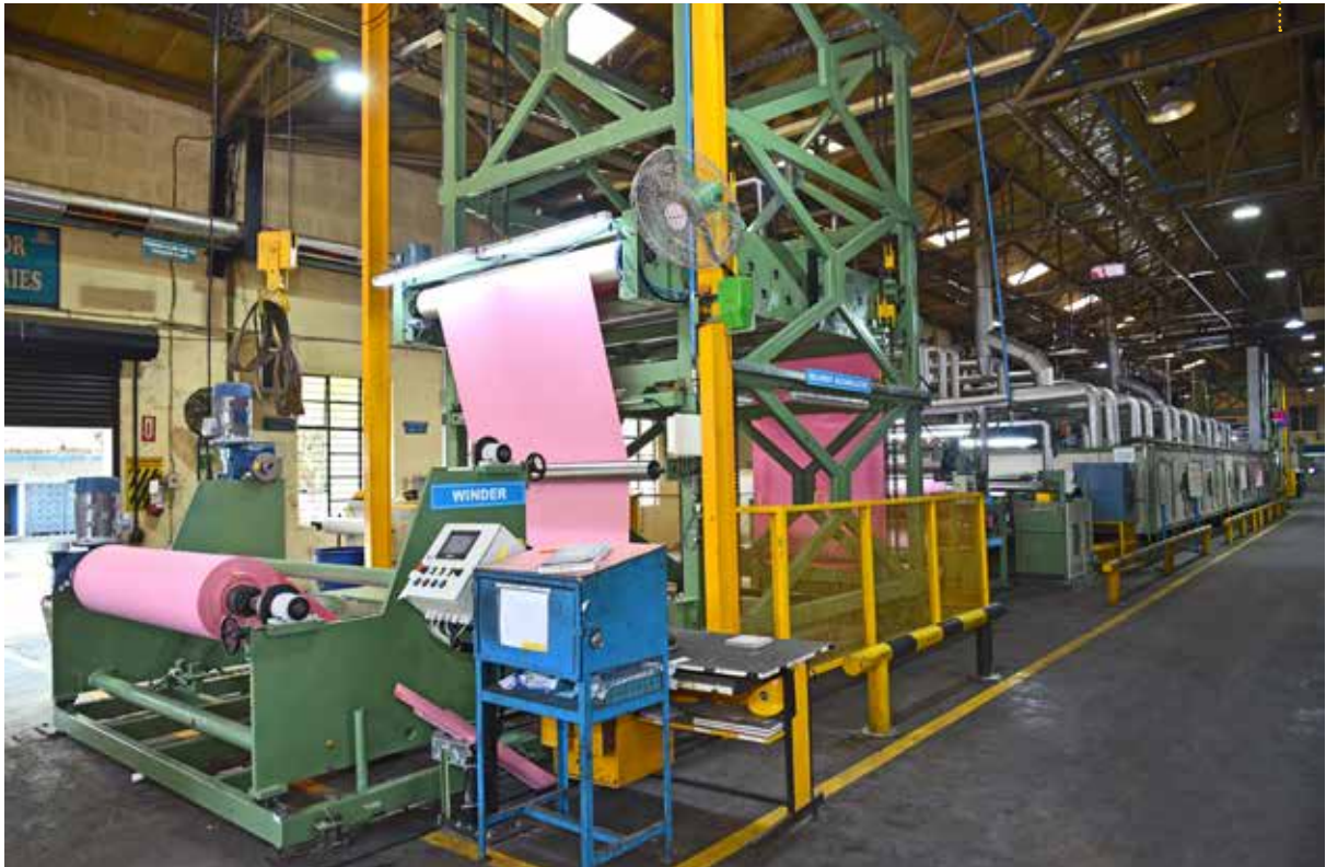
Stenter at Maraimalai Nagar, processes cloth backings for Coated Abrasives
