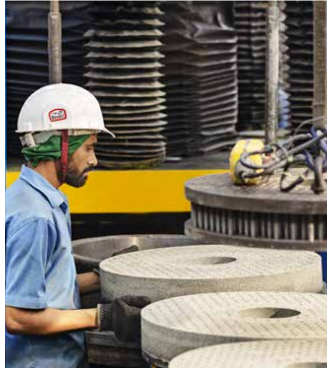
Manufacturing of precision resinous wheels for spring grinding
