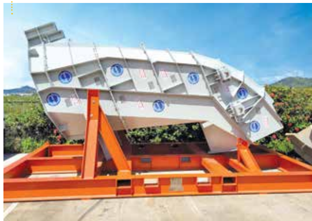
Stacker reclaimer bauxite soft loading chute – refurbished and lined with rubber/ceramic composite liners
