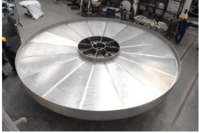
Continuous Pan Filter Germany
