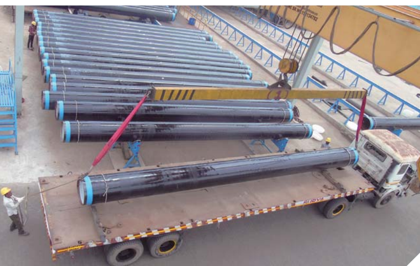
3LPE coated pipes at Anjar Plant, Gujarat
