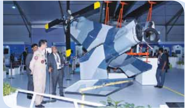
Naval Utility Helicopter demonstrating tail boom and main rotor folding during Aero India-2019.
