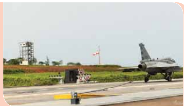
The LCA Naval Prototype 2 (NP2), safely executed the first contact of the arrestor hook system with Arresting wire at moderate taxi-in speeds on location at the Shore Based Test Facility, INSHansa, Goa, on 2 nd August, 2018.
