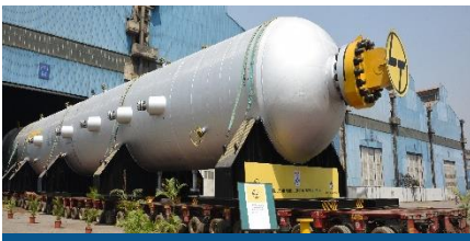
Hydrocracker, HPCL Visakh Refinery
