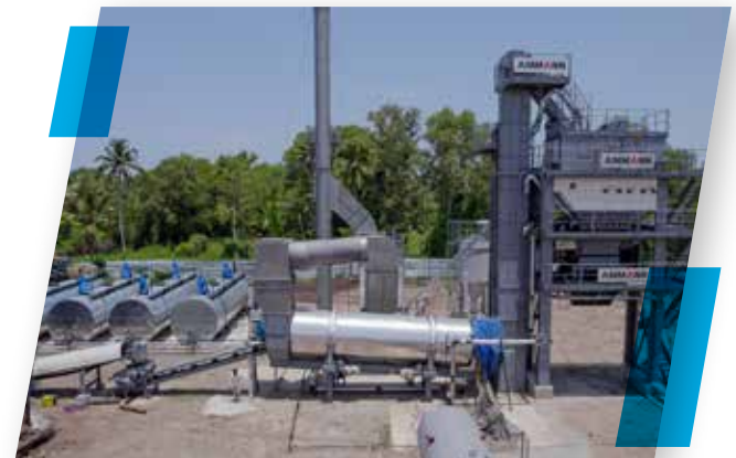
AMMANN VT-180 TPH HOT MIX PLANT
