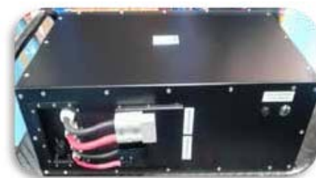
Golf Cart Battery Pack
