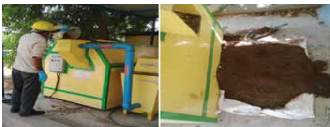
Automatic compost machine at Bawal
