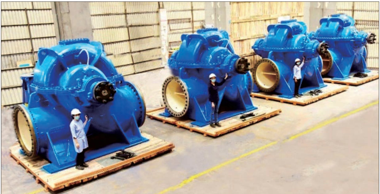
Largest Split-case Pumps supplied to UP Irrigation Department
