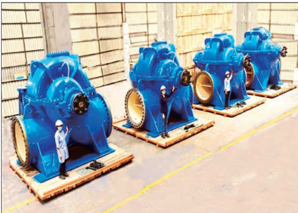
KBL has supplied and commissioned largest ever horizontal split case pumps across different locations of the Uttar Pradesh State Irrigation department (CESPO)
