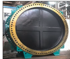
3800 mm diameter Butterfly Valve
