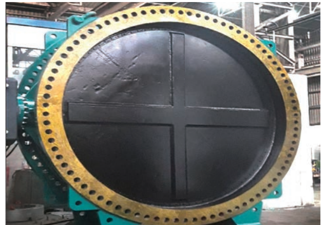
KBL has manufactured and supplied its biggest Butterfly Valve of 3800 mm diameter
