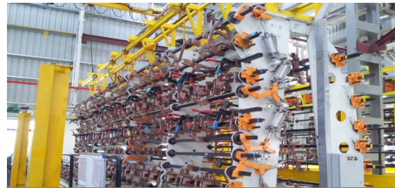
Bus Assembly Welding Fixture of size 12M
