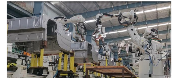
Indexing Arrangement for Spot Welding Line
