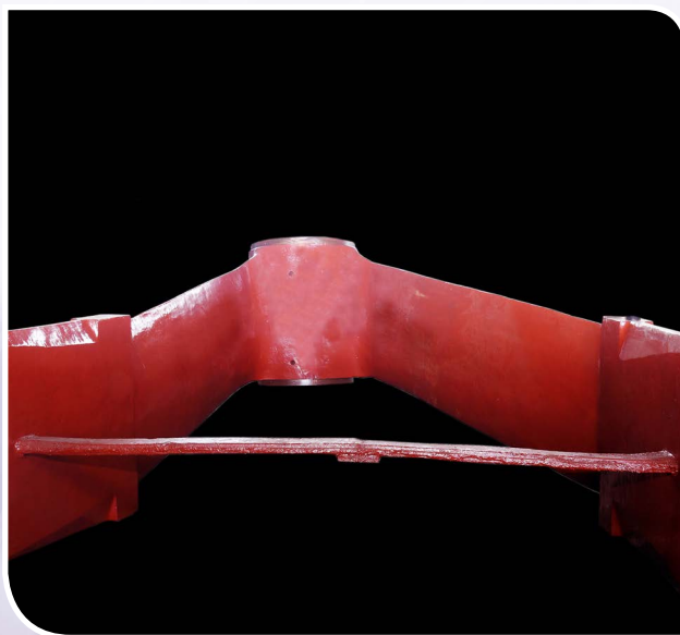
A-Bracket (AFT) for Marine application - 8.2 MT each
