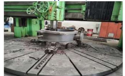
Machining of Valve outer casing.
