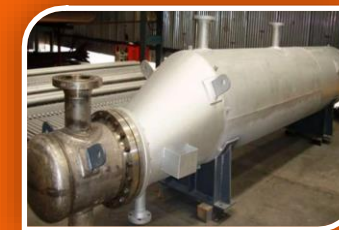
Co2 Solution Reboiler
