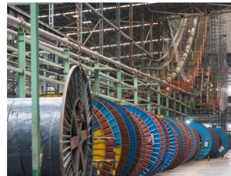
Catenary Continuous Vulcanizing lines
