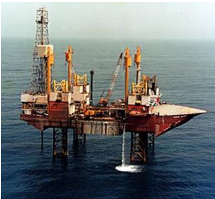
Sagar Samrat MODU being converted to MOPU
