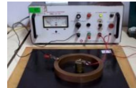
Electrical Resistance Test
