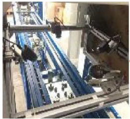
Vision Camera for Thrust washer - Pokayoke
