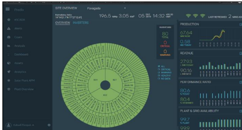
Real Time Dashboard at CCRA / Remote Console used for Predictive Analysis, Scheduling & Forecasting
