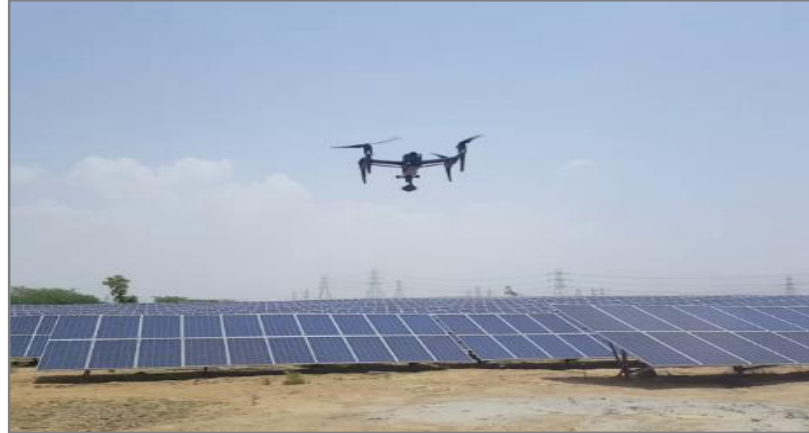
Use of Drones for detecting offline strings, hot spots, diode faults, reverse polarity, string mismatch, micro cracks & surface faults.
