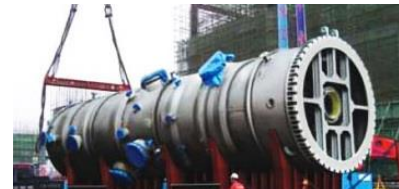
Coal Gasifier for China
