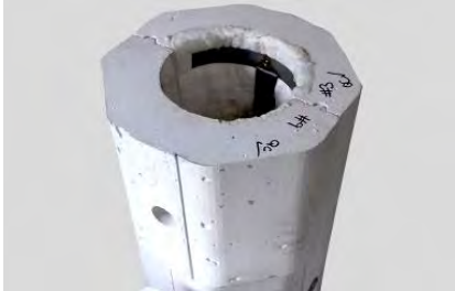
Precast Skid Pipe Cladding
