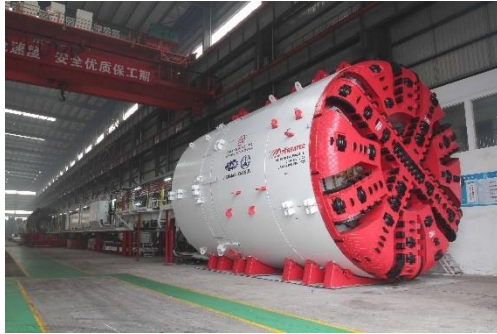
Tunnel Boring Machine (TBM)
