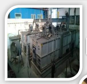
Spherodizing & Annealing Machines
