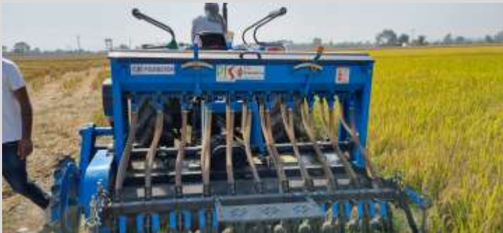
A Happy Seeder machinery donated by PFS (to farmers Coop Societies) in operation in the fields of Ludhiana. No stubble burning by farmers after use of the machines.
