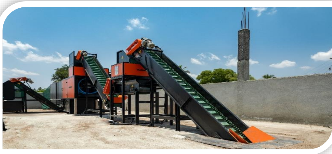
Waste Management via TRASHBOT - A de-centralised Automated Mixed Waste Segregator
