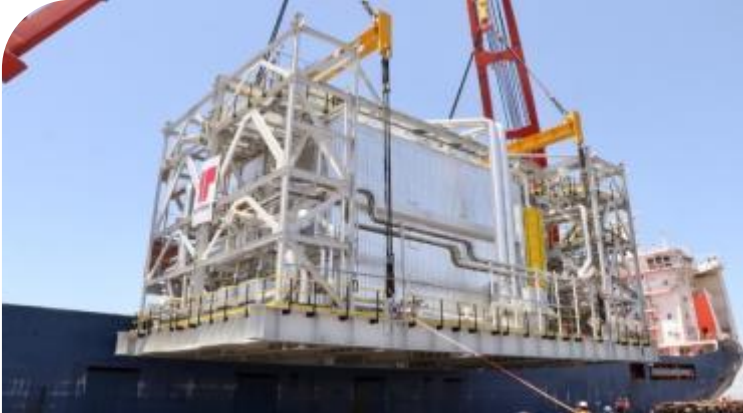
Two units of modularised plug and play boilers shipped to the Middle East
