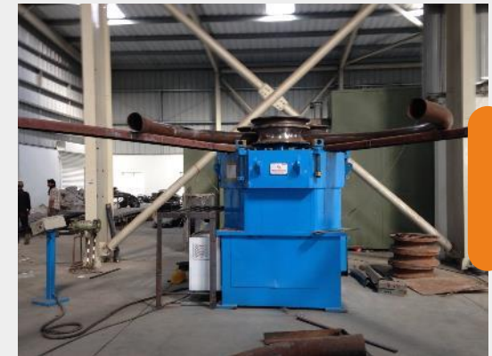
Pipe Rolling Machine pto Ø200 X 8 Mm
