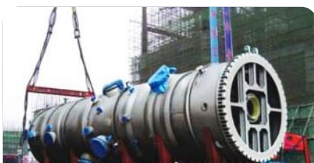
Coal Gasifier for China
