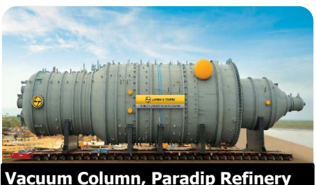
Vacuum Column, Paradip Refinery
