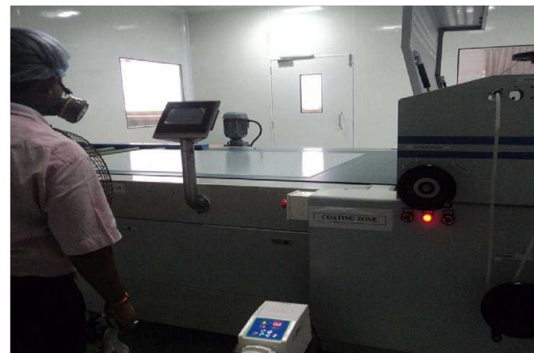
AR COATING PROCESS IN A CLEAN ROOM
