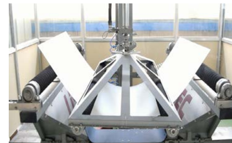
Withstood > 180 Mpa (Standard 90 Mpa as per EN 12150-1)
