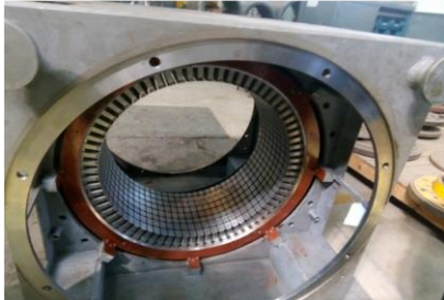
HYDRO GENERATOR UNDER ASSEMBLY FOR SUNDARIJAL HYDRO PROJECT, NEPAL
