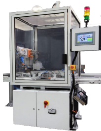
Keyence Camera System for Automatic Inspection
