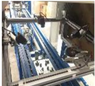
Vision Camera for Thrust washer - Pokayoke
