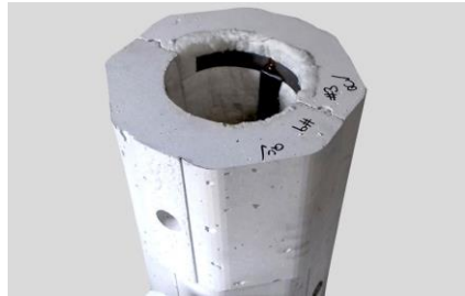
Precast Skid Pipe Cladding
