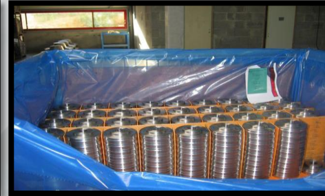
Application for Anti-Corrosive VCI Material
