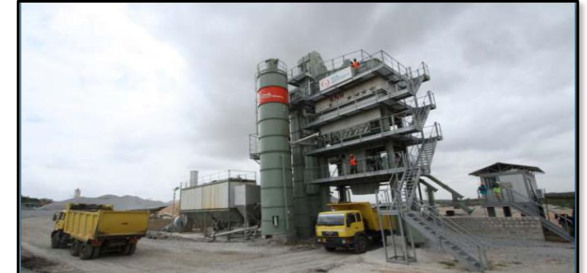
240 TPH D & G Hot Mix Plant
