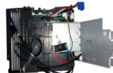
ODU Inverter Control Box
