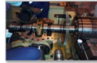
228MW, STEAMTURBINE,SABIYA, KUWAIT, MAIN OIL PUMP OVERHAULING
