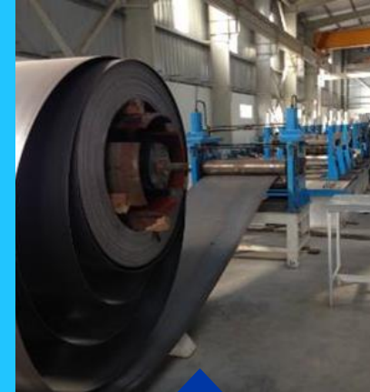
Pipe Rolling Machine pto Ø200 X 8 Mm
