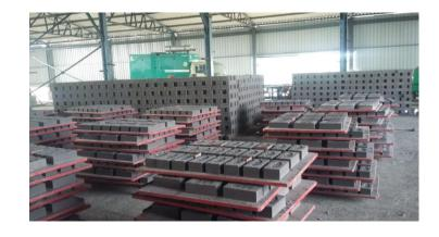
Fly ash bricks which are manufactured from various industrial wastes such as fly ash, sand, stone, dust and cement, are used globally nowadays over clay bricks and traditional red bricks
