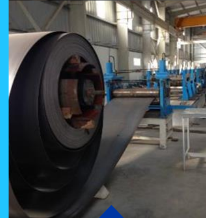
Pipe Rolling Machine pto Ø200 X 8 Mm
