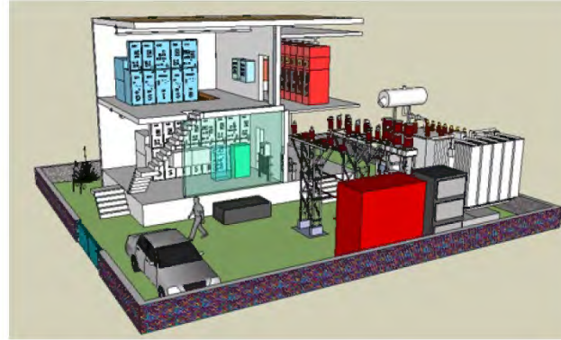
Compact 33 kV Distribution Station
