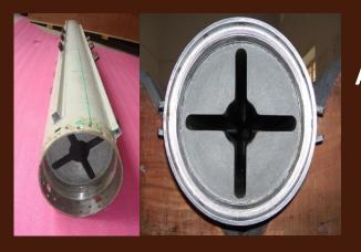
**Astra Motor cast with Smoke-less Propellant**
