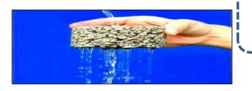
Perviouscrete<sup>™</sup> is "Rain water harvesting" concrete.
