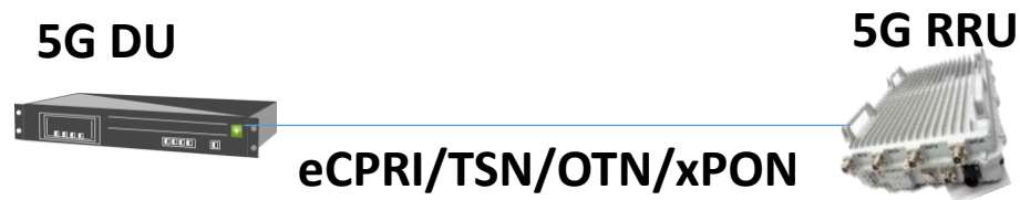
Multi-protocol support to deliver comprehensive 5G front-haul solutions
