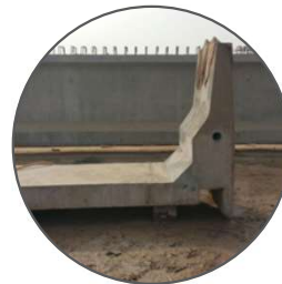
Fabricated Casting Panels and Moulds
