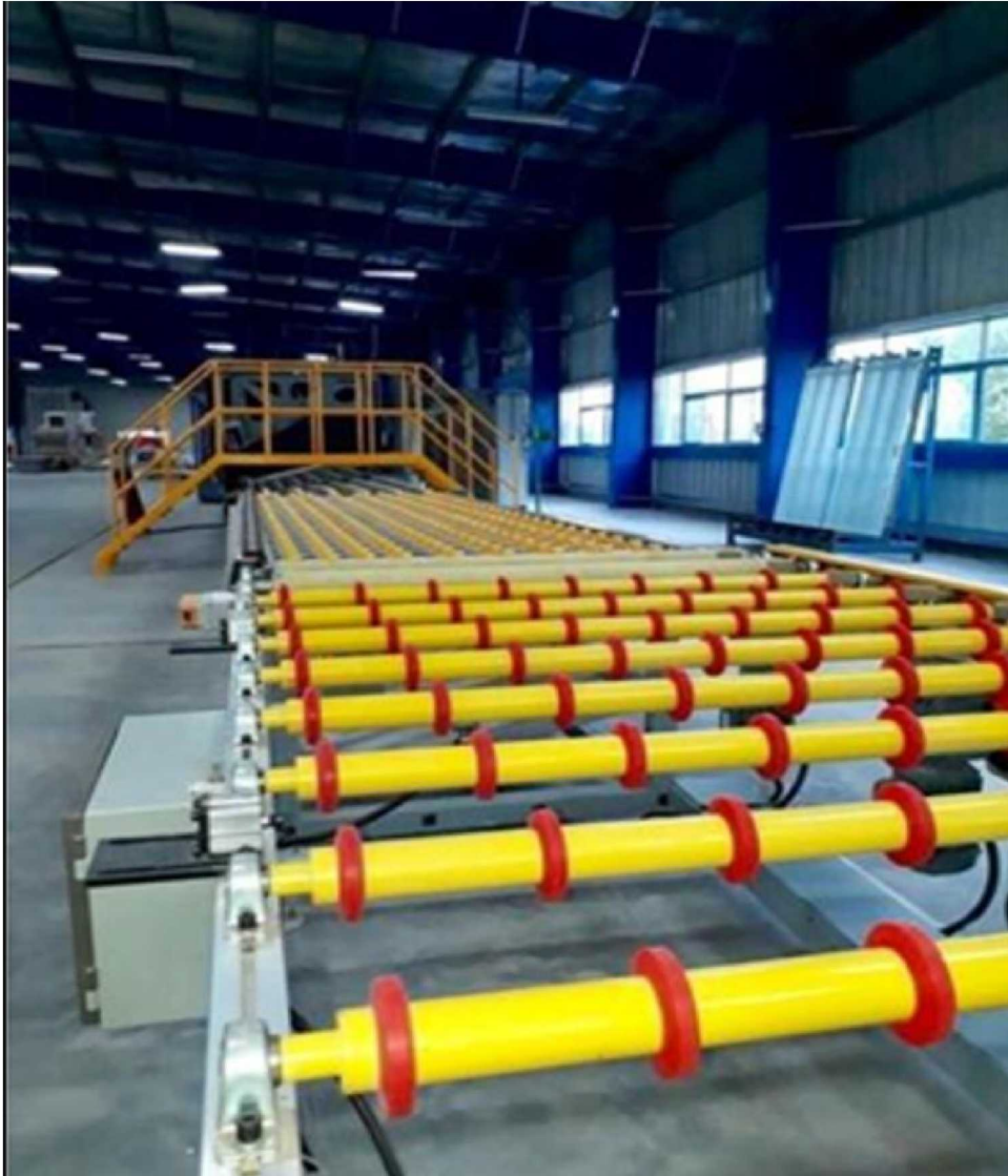
Trend setting European technology that fully tempers glass which floats on an air cushion
