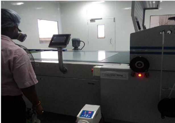
AR Coating Process in A Clean Room
