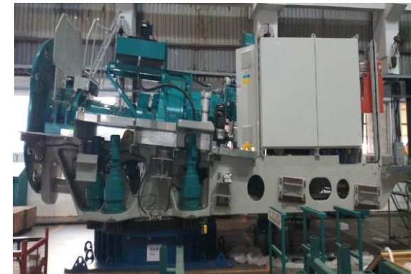
S120 Nacelle Assembly at Plant
